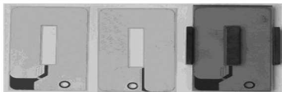
Fig. 2.8. Secondary windings (a) Secondary windings of the test ICT.
